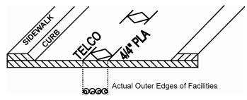
d. Corridor Marking: Used to mark multiple facilities of the same type (e.g., electric), bundled or intertwined in the same trench, where the total number of facilities is not readily known (operator has no record on file for the number of facilities). Marks are placed over the approximate center of the facilities and indicate the width of the corridor. The width of the corridor is the distance between the actual located outside edges of the combined facilities.
