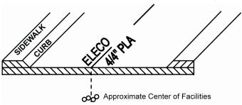
c. Conduit Marking: Used for any locatable facility being carried inside conduits or ducts. The marks indicating the outer extremities denote the actual located edges of the facilities being represented.
