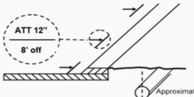
Used when marks cannot be placed directly above buried facility.
